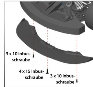
**Installation des 160 km/h (100 mph) Splitters**
