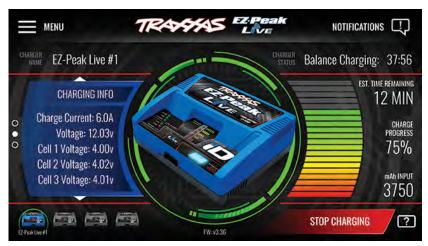
Charge Dashboard - Follow the progress of the connected battery with this intuitive status screen. Monitor cell voltage, view estimated time remaining, and even track charge current all in one convenient view.
