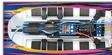
The integrated battery trays secure a wide variety of battery packs from 8.4V NiMH batteries all the way up to 8400mAh 3s LiPo packs. A high-output TQi 2.4GHz radio with the innovative Traxxas Stability Management (TSM) system keeps Spartan under complete control as it slices through the water. Spartan delivers the power, speed, convenience, and fun for which Traxxas' award-winning cars and trucks are known. Prepare yourself for the ultimate RC boating power trip, only from Traxxas.
