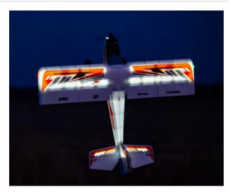
The E-flite® Night Timber® X 1.2m adds an integrated high-intensity LED lighting system to the 3D and STOL-capable Timber® design so you can fly all day AND all night, too! It's also Smart Technology ready with a Spektrum™ Avian™ 60-amp Smart ESC installed (along with an AR637TA receiver in the BNF Basic version).
