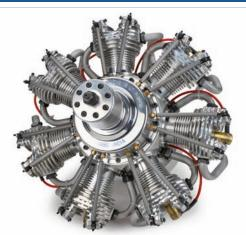
This is one of the worlds smallest available 7 Cylinder radial engines, completely CNC machined from solid aluminium. The miniature parts are made to the highest exacting tolerances resulting in a very smooth running engine.
