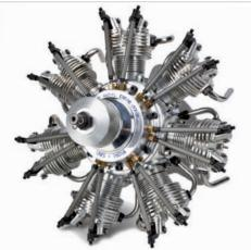
All components of this fine engine are newly developed, and it features a crankcase made of aero grade aluminium, high quality aluminium casting cylinder heads in a natural colour, and an open valve drive with long push rods.
