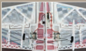
Carbon verstärkter Rumpf carbon-reinforced foam airframe
