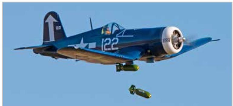
Payload Release Unit clearly shown mounted to the new Hangar 9 60cc Corsair.
