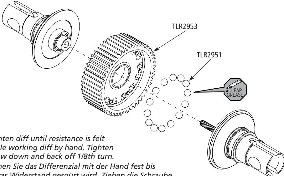
**EN** Tighten diff until resistance is felt while working diff by hand. Tighten screw down and back off 1/8th turn.
