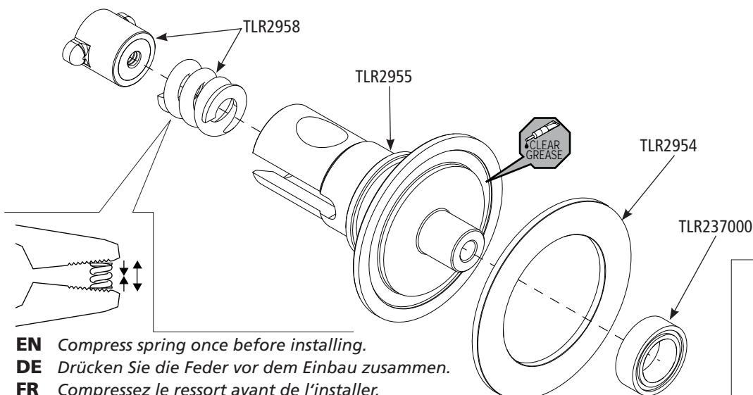
**EN** Compress spring once before installing.
