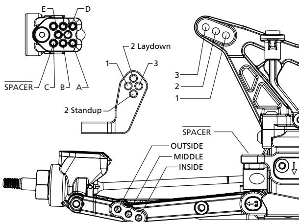
**Rear Suspension**Configuration:  Laydown  StandupLD Diff. Height:  Standard  +3.5mmTransmission Type:  3-Gear  4-GearToe Inserts:  0.5  1  1.5  2  2.5  3  3.5  4Anti-Squat Inserts:  0  0.5  1  1.5  2  2.5  3Inner Roll Center:  LRC  HRC
