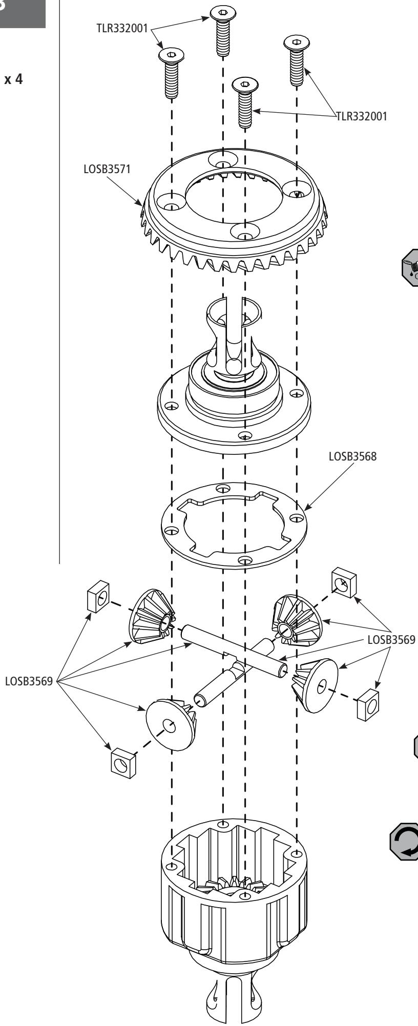
**EN** Fill with 7000cs oil just above the planetary gear.
