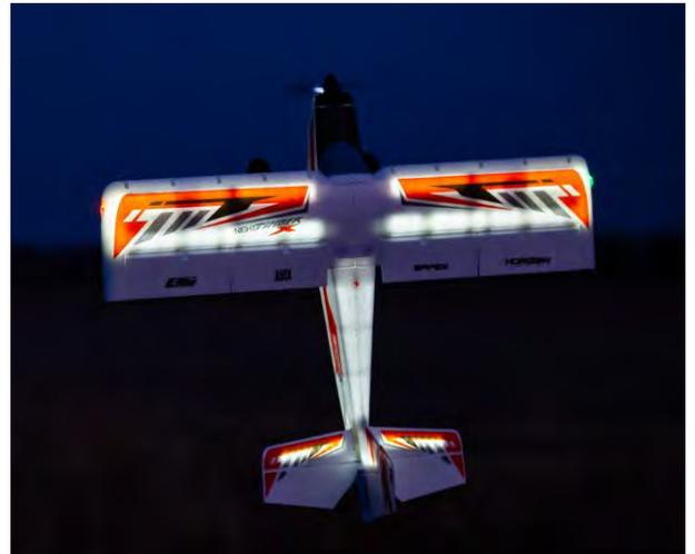
The E-flite® Night Timber® X 1.2m adds an integrated high-intensity LED lighting system to the 3D and STOL-capable Timber® design so you can fly all day AND all night, too! It's also Smart Technology ready with a Spektrum™ Avian™ 60-amp Smart ESC installed (along with an AR637TA receiver in the BNF Basic version).
