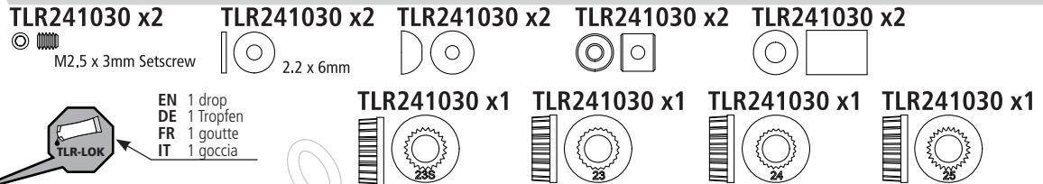
**EN** Use correct insert for servo spline.
