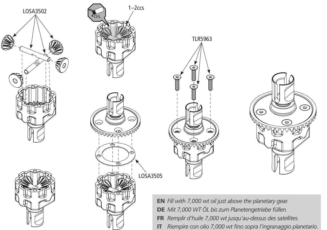
**EN** Fill with 7,000 wt oil just above the planetary gear.
