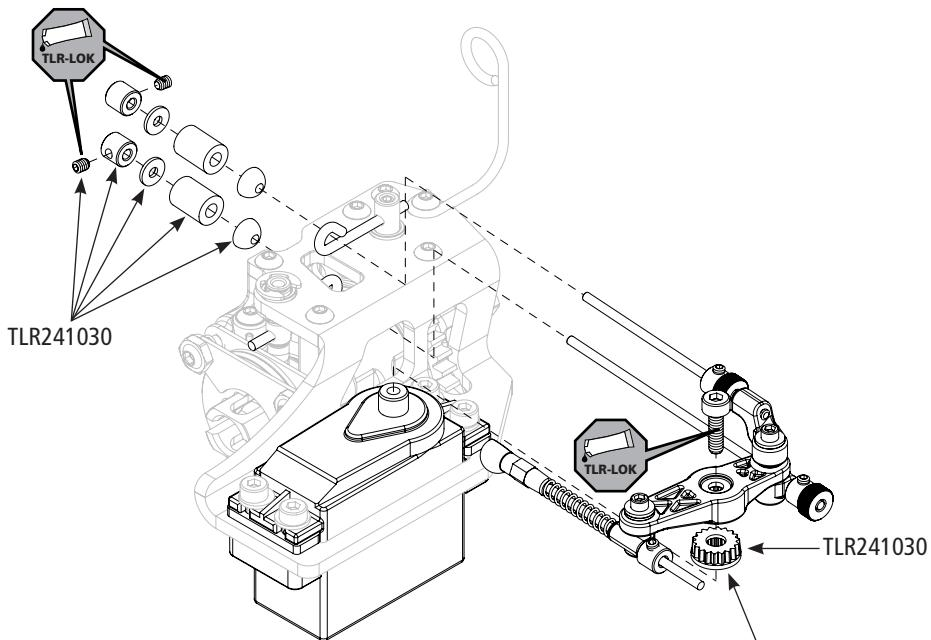
**EN** Use correct insert for servo spline.
