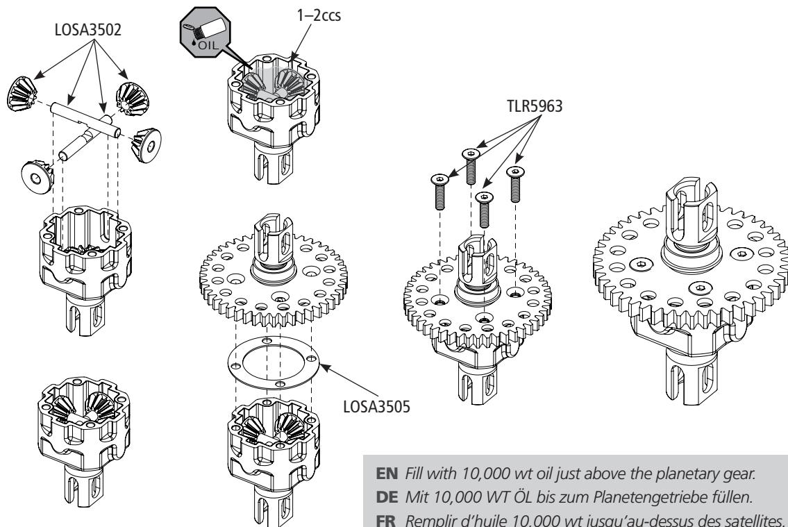
**EN** Fill with 10,000 wt oil just above the planetary gear.
