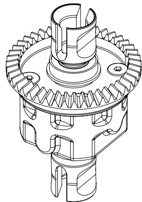
**EN** Fill with 4,000 wt oil just above the planetary gear.
